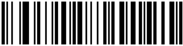
ITF25 Turn On Check Bit and does not send
