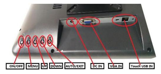
• TOUCH USB: this is connected to PC's USB Ports, used for touch function
